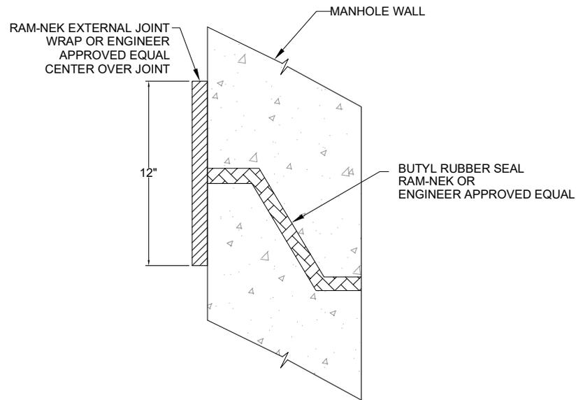
MANHOLE JOINT DETAIL
