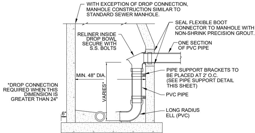
\*DROP CONNECTION REQUIRED WHEN THIS DIMENSION IS GREATER THAN 24"
