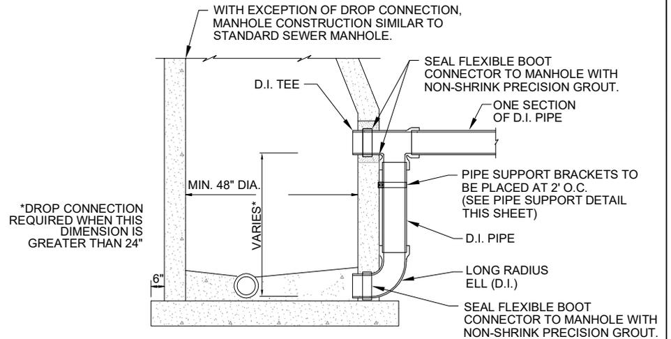
\*DROP CONNECTION REQUIRED WHEN THIS DIMENSION IS GREATER THAN 24"
